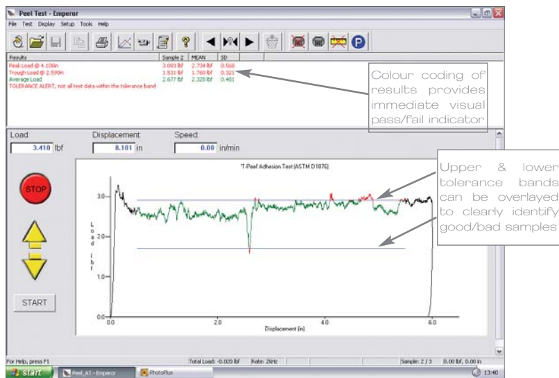
Tolerance band facility
