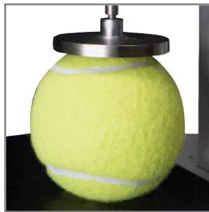
Tennis ball compression test
