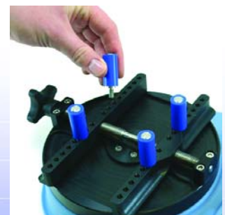
Gripping pegs are easily adjusted to match sample dimensions.
